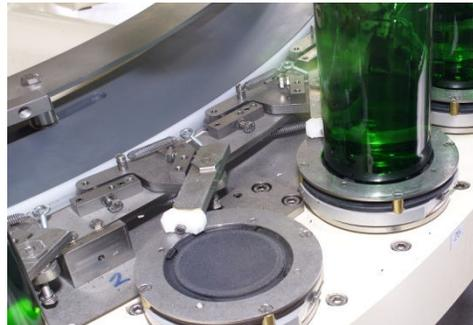
Photo 4: Mechanical Orientation for Side-wall Lug
